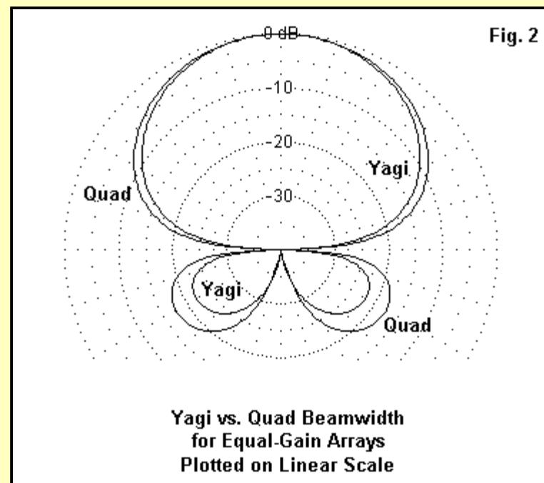
**2. Quad vs. Yagi beamwidth:** At every level sampled where the gain of a quad array could be roughly equated with the gain of a Yagi array, the quad exhibited wider -3 dB and -0.5 dB beamwidths. As shown in **Fig. 2**, the difference is most dramatic at lower gain levels: the plots show antennas with 7+ dBi free-space gain levels. The linear plot is necessary to display the two patterns clearly.
